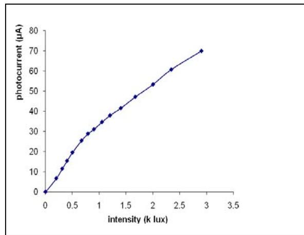
Fig. 3 Photocurrent with various light intensities.
