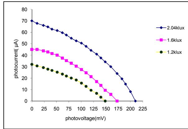
Fig. 2. I-V Characteristics of CdS-Cu<sub>2</sub>S Cell with Various Light Intensities
