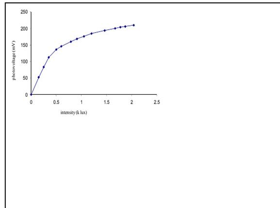
Fig. 4. Photovoltage with various light intensities.
