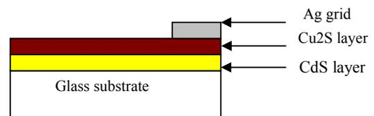
Fig.1. A schematic cross section of CdS-Cu<sub>2</sub>S photovoltaic cell
