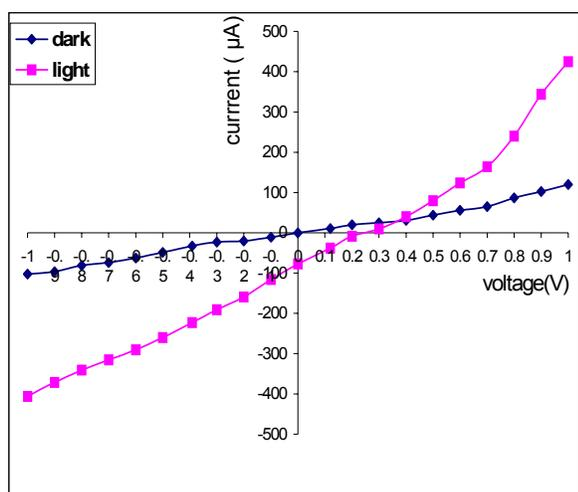
Fig.5. I-V Characteristics of CdS–Cu<sub>2</sub>S Cell
