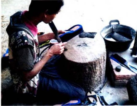
Figure (24) Making the *pontaw wet-htaukatipa* slipper
