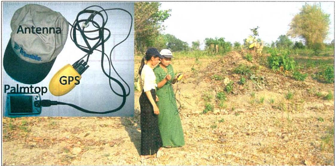
Photo (1) Mapping matpe field by using GPS (upper left photo shows the GPS used in mapping)
