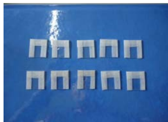
Figure 10(b) Preparation of glass with masking tape
