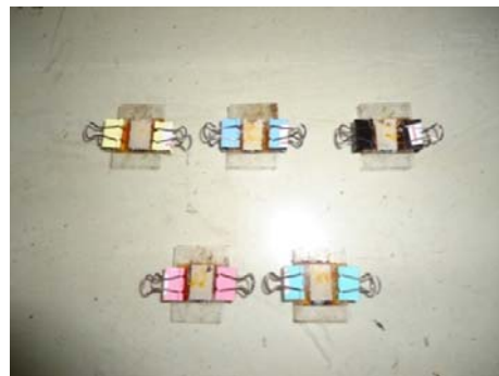
Figure 14. DSSCs with binder clips
