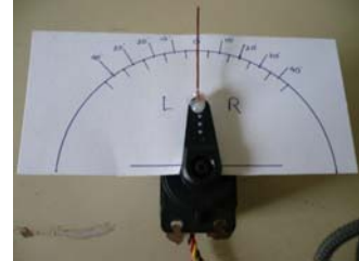
Fig. 3 Servo motor at central position (0 degree)
