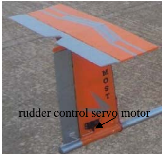
Fig. 5 Servo motor mounted on rudder control surface
