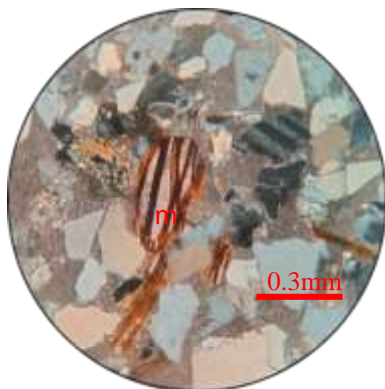
Figure (8) Biotite mica(m) show bifurcated structure by the replacement of calcite cement in sandstone of the Moza Formation (XN)
